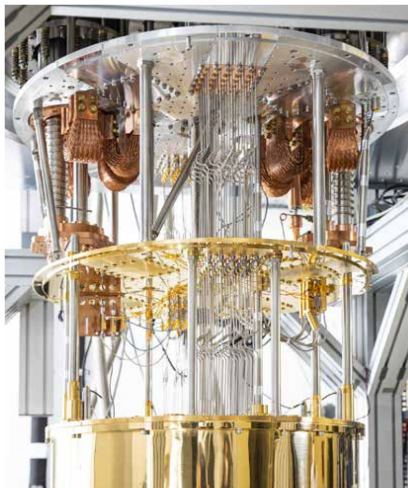
Cryogenic setup and control of a superconducting quantum computer at Forschungszentrum Jülich
