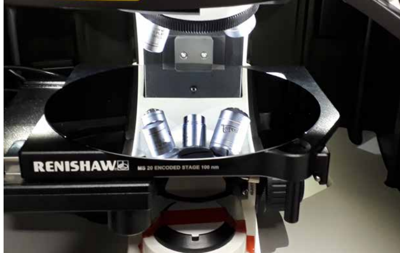
Analysis of a 200 mm Si wafer with 100 nm positioning accuracy
